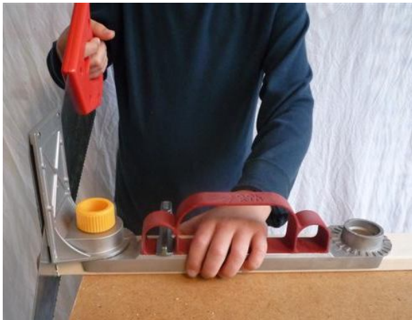
holder with brace and 2 fastening points
